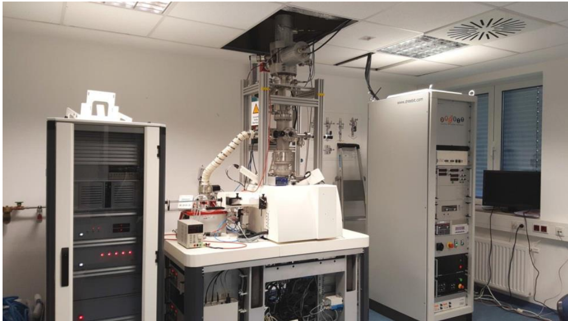
Figure 3: Overview photograph of the system for deterministic single ion implantation as built in the Leibniz Joint Lab “Single Ion Implantation” located at the IOM in Leipzig.
